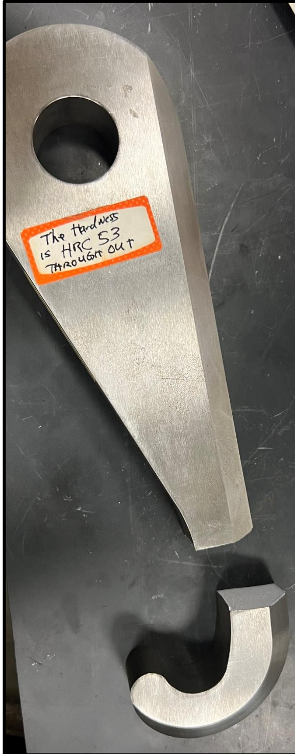
Figure 4: Asymmetrical loading fixture hook failure
